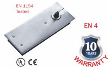
AVFS 844 Floor Spring (Door Weight 150kg) Max. Door Width 1100mm,
