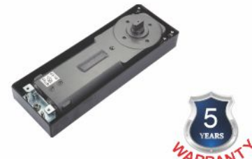
AVFS 943 Floor Spring (Door Weight 120kg) Max. Door Width 1050mm, Cover Plate Finish - SSS
